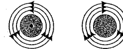
A dot in the center of the wire indicates electron flow out of the plane of the page, toward the reader. An "x" in the center of the wire indicates electron flow into the plane of the page, away from the reader.
